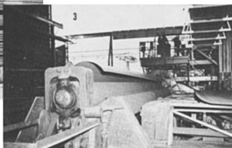
In 1947, the trans-Arabian pipeline was started. Thousands of tons of steel plate were fabricated into 31 foot lengths of pipe at factories in the United States.
