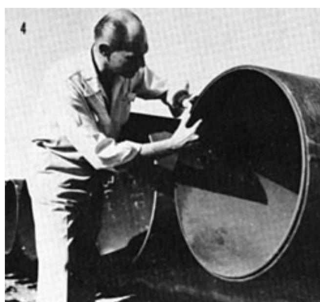
Half the pipe was made 30 inches in diameter and the other half 31 inches. This made it possible to save shipping space by "nesting" or slipping the smaller pipe inside the larger.
